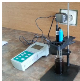
Fig. 4. Examining the alkalinity of finished products at PH-150 MI (Ukraine)
