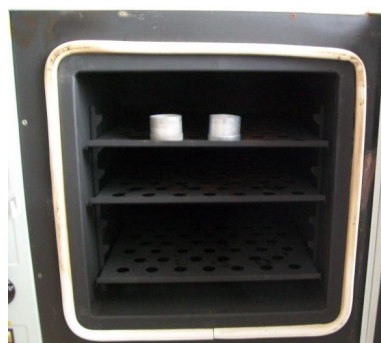
Fig. 3. Drying cabinet for measuring the moisture content of finished goods SNOL (Ukraine)
