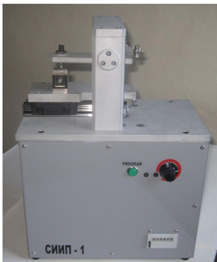
Fig.3. General view of test stand СИИП-1 for wear resistance.
