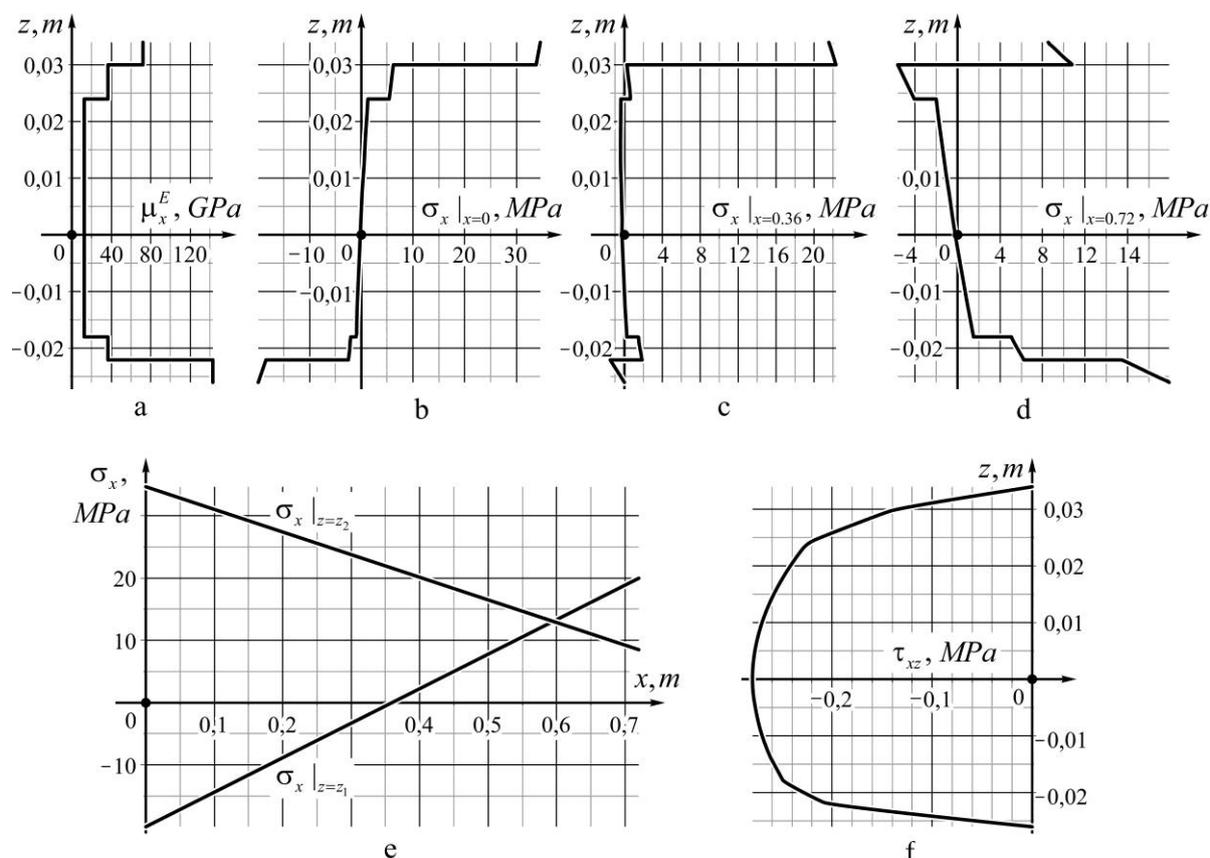
**Figure 4.** Graphs of normal and shear stresses.
