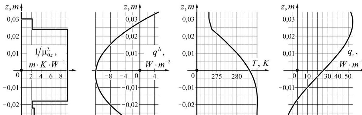
**Figure 3.** Initial data and results of solving the heat conduction problem
