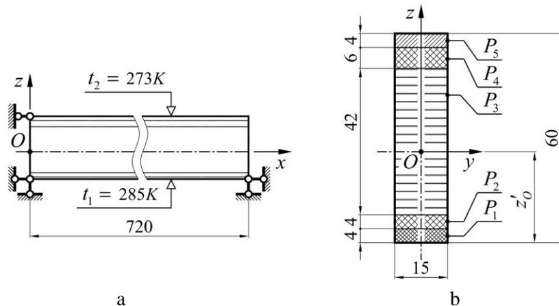
**Figure 2.** The scheme of kinematic restrictions and the cross-section of the beam (dimensions in mm).
