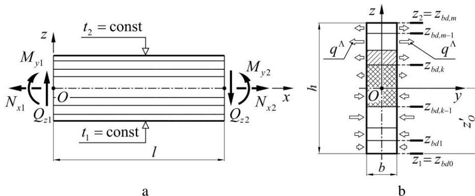
**Figure 1.** Scheme of a section of a bar and its cross section.
