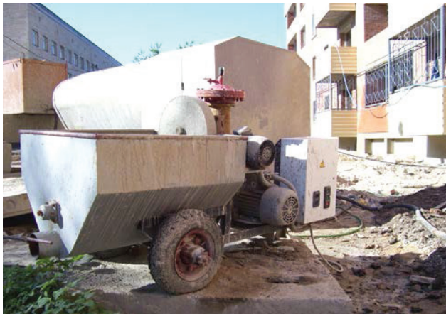
Fig. 3. Production testing of one-piston mortar pump RN-3.8 with universal mortar mixer URZ-3.8 (building site of company «Poltavtransbud»: Alexander Bedniy Street, 3a, Poltava, Ukraine)
