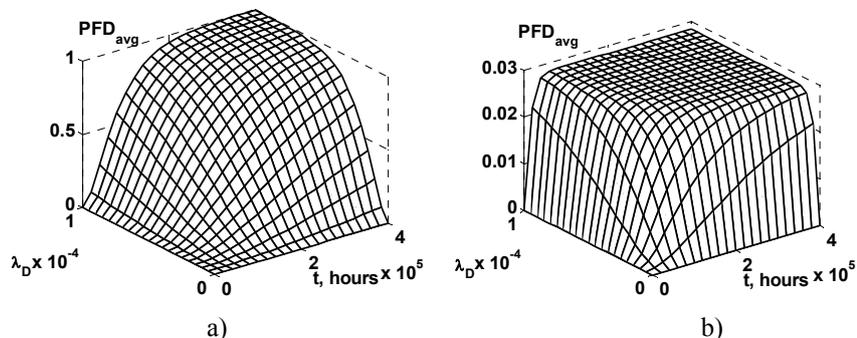
Fig. 9. Dependence of  $PFD_{avg}(t)$  function behavior from the input parameter  $\lambda_D$  for MSaf1 (a) and MSaf2 (b)
